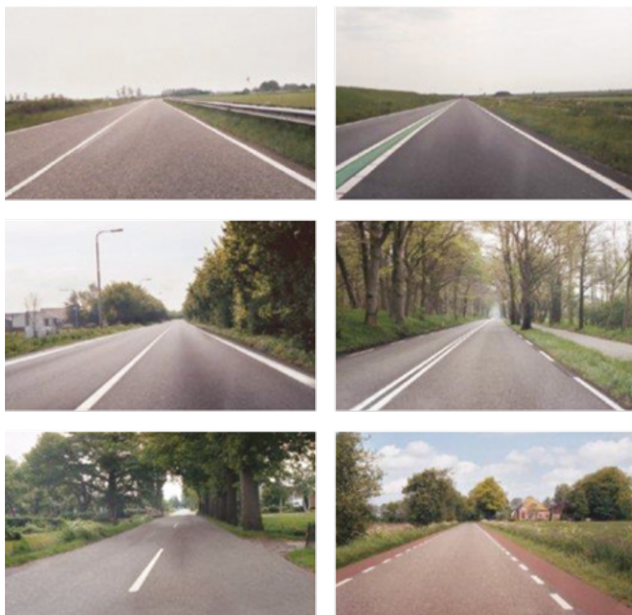
Illustration 53: Traditional road layout and road layout according to the guideline 'essential recognisability characteristics' for the three sustainable safe road categories. As implementation of ERCs has particularly taken place on rural roads, only rural road variants are shown
