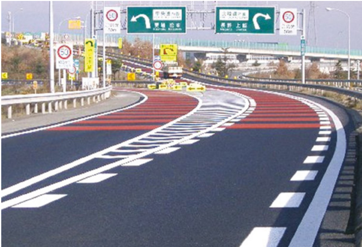
Illustration 19: The lane diverging to the right has signage indicating it bends to the right, and the road in distance reinforces this perception, however, the road veers to the left before sharply veering to the right.
